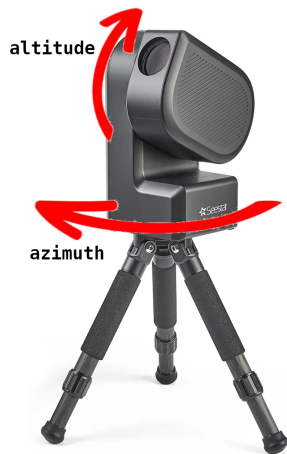
Figure 1: Seestar S50 in alt-azimuthal mode.
