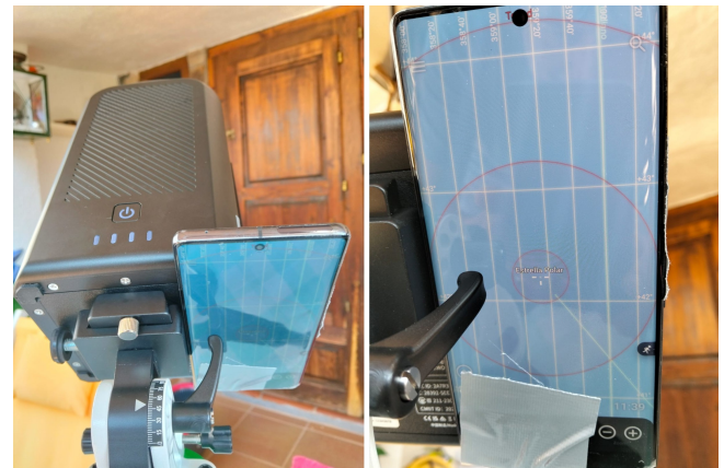
Figure 6: Mounting the smartphone-Seestar system to point to the North Star
